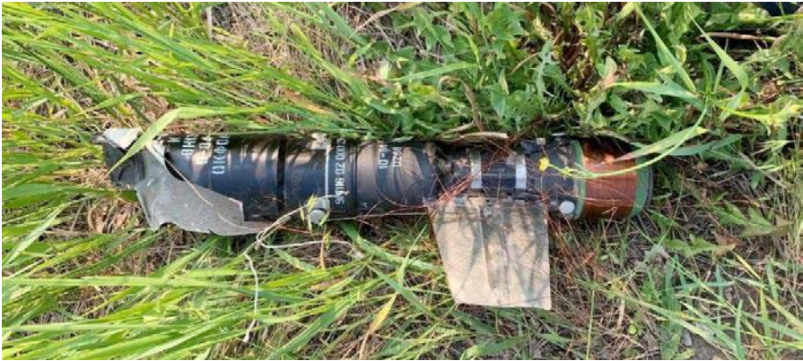
Motor section of fired 9M116. Image © SESU
